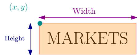
Figure 2.3: The position of section titles and other zone “boxes” can be identified using (x, y) , width and height attributes. This allows for easy cropping.
